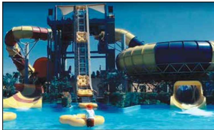
The bowl slide and tornado both utilize four-person rafts and share the same lift system. COURTESY AQUA PLANET
