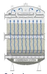
**Backwash**REDUCES BACKWASH WATER 60% BY WASHING 2 SF OF FILTER MEDIA AT 15 GPM/SF RATE
